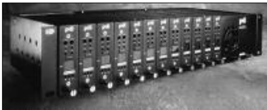
Twelve PDI-50121AD demodulators in housing
